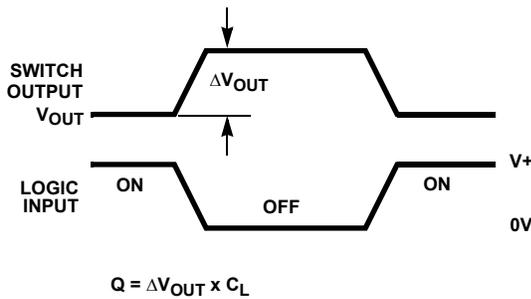
$$Q = \Delta V_{OUT} \times C_L$$
