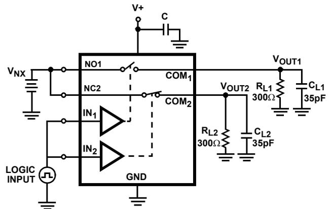
$C_L$  includes fixture and stray capacitance.
